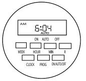
The 24 hour digital timer with 1 minute intervals will display the current time when operating. it will control eight (8) separate timing programs. There are many combinations of timing available to the user. Such as: hourly, daily, or weekly settings. NOTE: We recommend that you plug in your timer in for approximately 3 hours before programming to charge internal battery.
