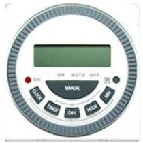
The 24 hour digital timer with 1 minute intervals will display the current time when operating. it will control eight (8) separate timing programs. There are many combinations of timing available to the user. Such as: hourly, daily, or weekly settings. NOTE: We recommend that you plug in your timer in for approximately 3 hours before programming to charge internal battery.
